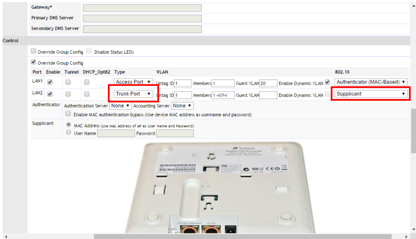
FIGURE 21 Configuring an AP Ethernet port as an 802.1X Supplicant
